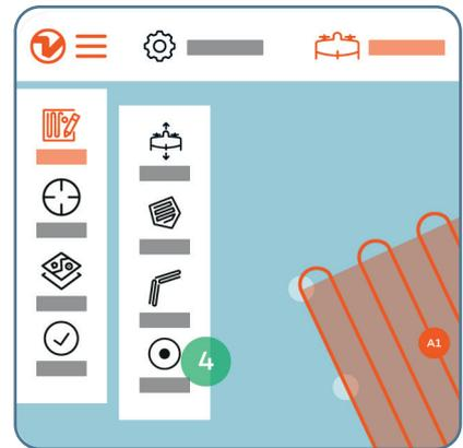
4. (Optional) loiter waypoints are automatically inserted between two areas; additional waypoints can be inserted manually to ensure safe flight paths between areas and back to the home point
