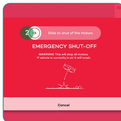
As the last option in dangerous situations, it is possible to immediately switch off the motors of WingtraOne at any time in-flight.
